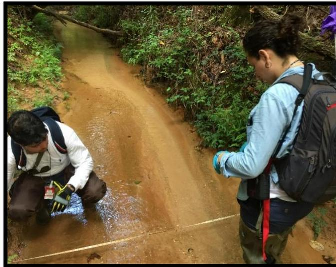
Figure 15: Measuring the stream width manually
