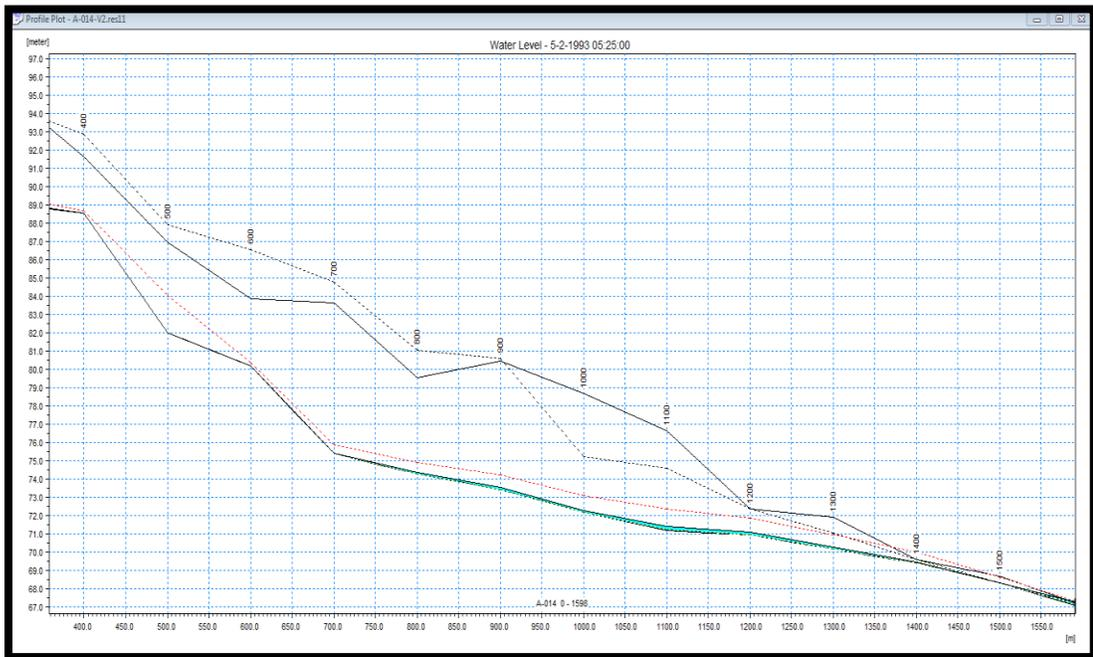
Figure 43: Water level along A-014 (February) without culvert and weir
