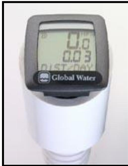
Figure 9: FP101 Global Water flow meter ("FP101 & FP201 Global Water Flow Probe," 1990)
