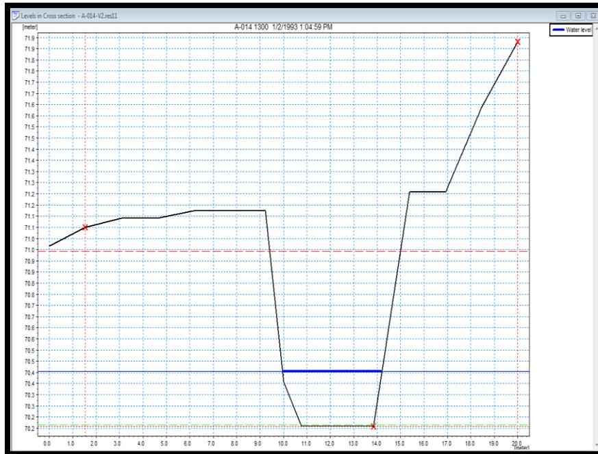
Figure 39: Water level at cross-section without the culvert and weir (1300 m from outfall)
