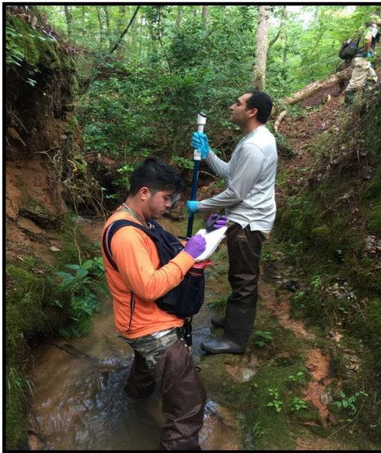
Figure 10: Measuring water velocity in the A-014 stream at SRS during summer 2016
