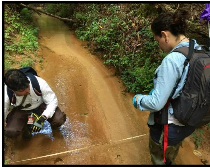
Figure 15: Measuring the stream width manually
