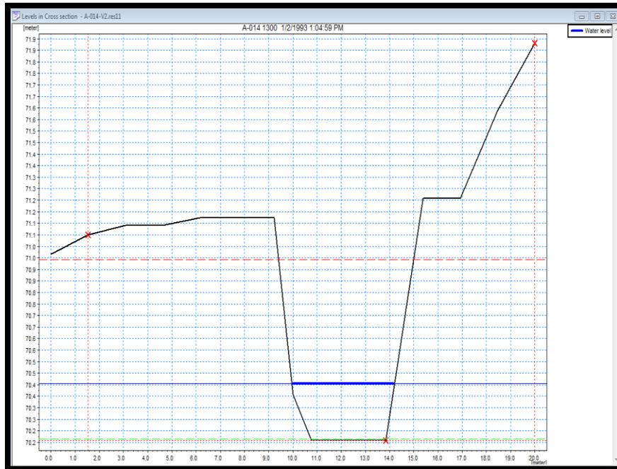
Figure 39: Water level at cross-section without the culvert and weir (1300 m from outfall)
